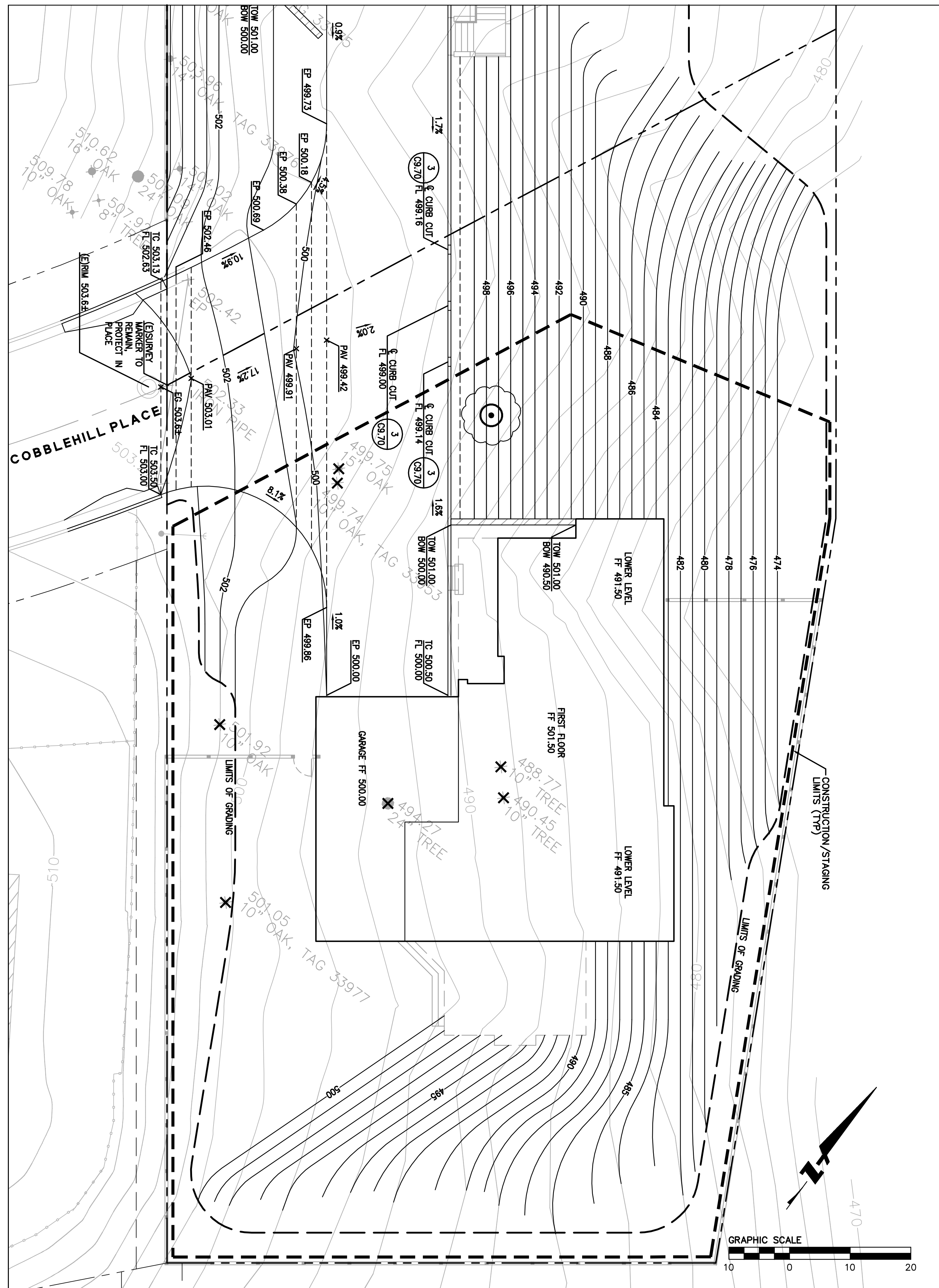
LOT 9 CLEARING, CONSTRUCTION, AND GRADING PLAN SCALE: 1"=10'
