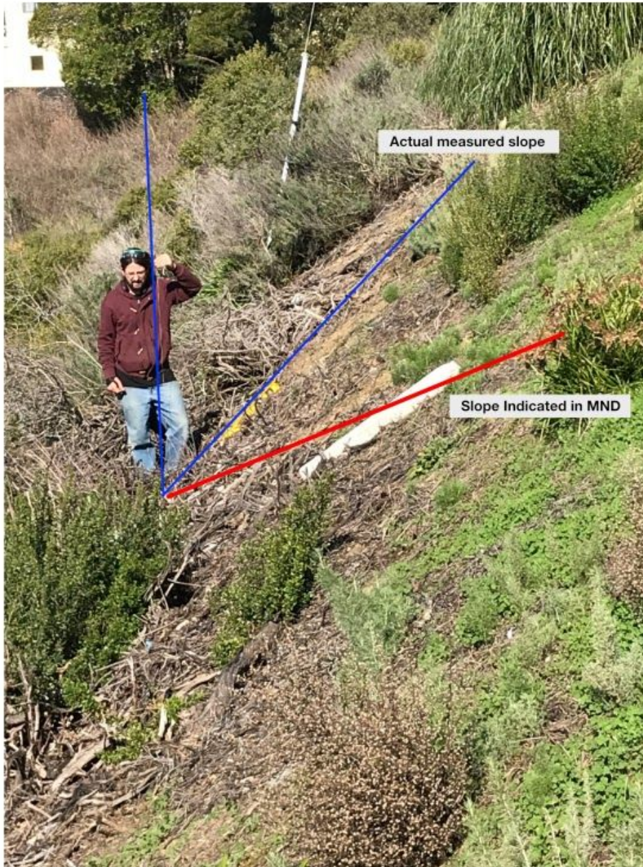
Figure 2 - Demonstrates in a simple way the difference between the mentioned 37% (the red line) to the actual slope (the blue diagonal line).
